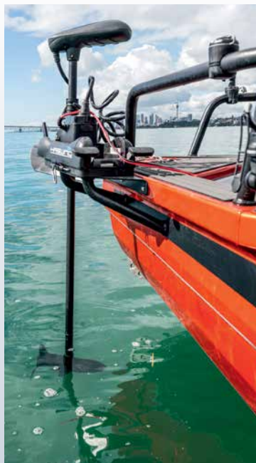
ABOVE A Haswing electric trolling motor is mounted on a custom bracket.
