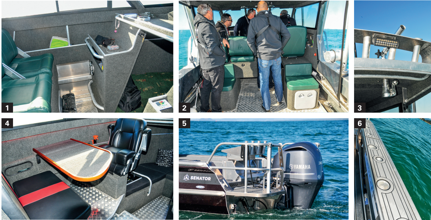
1) There are plenty of storage options in Bad Jelly; 2) Bad Jelly's seating includes a swivelling helm seat, two rear facing bench seats and two reversing bolster passenger seats; 3) The Rupp outrigger base is fitted through the hardtop; 4) The enclosed wheelhouse on Cousin Itt features a table, bench seat and reversable passenger seat; 5) A single 300hp Yamaha outboard powers Cousin Itt; 6) Four rod holders and three cup holders are set along each side.
