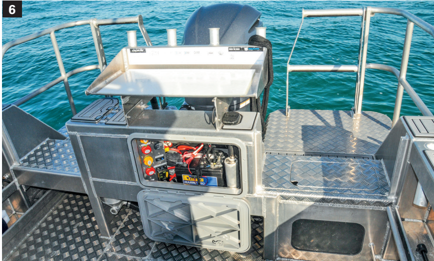
5) A wide beam and pontoon construction gives excellent stability; 6) Cousin Itt has two transom step-throughs and two batteries in the transom wall; 7) Both 780's have a heap of cockpit space, and Cousin Itt's features a customised Icey-Tek.
