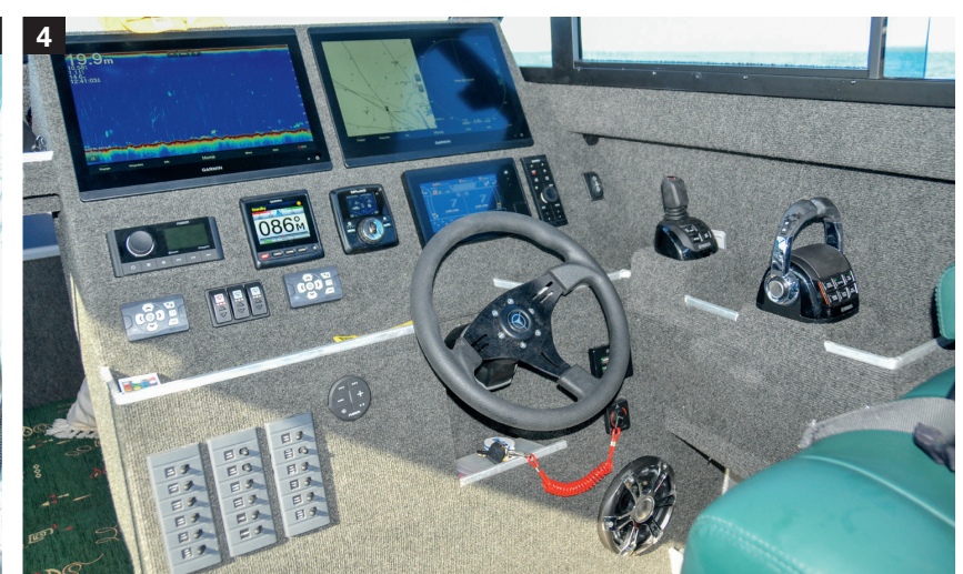
1) Cousin Itt heads out over the Bowentown Bar; 2) The pontoons help turn down the spray; 3) King and Queen helm seating on Cousin Itt; 4) Bad Jelly's helm controls feature a joy-stick control and twin binnacle.
