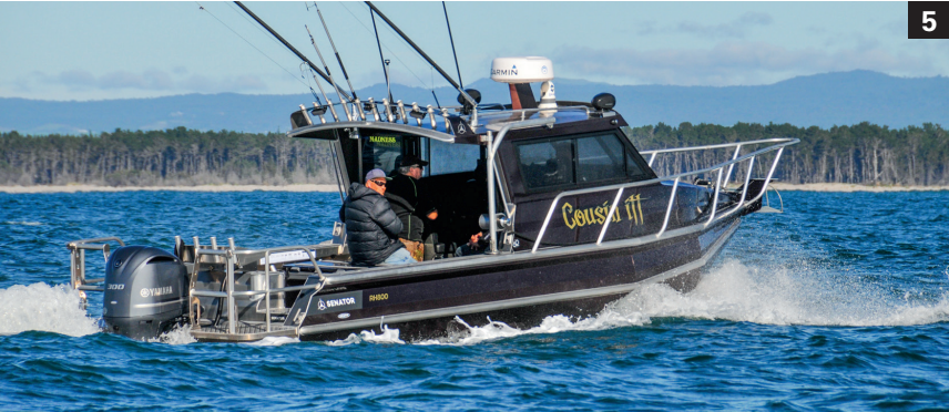
5) A wide beam and pontoon construction gives excellent stability; 6) Cousin Itt has two transom step-throughs and two batteries in the transom wall; 7) Both 780's have a heap of cockpit space, and Cousin Itt's features a customised Icey-Tek.
