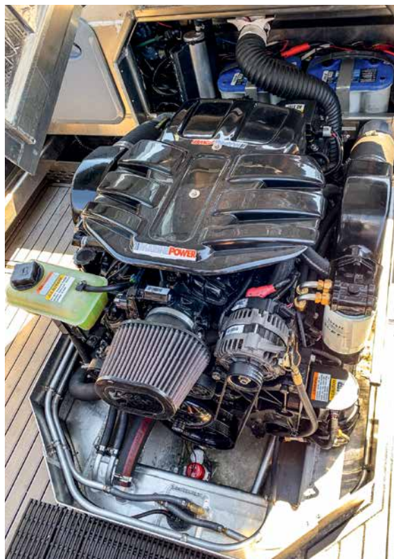
ABOVE The Marine Power Chev V8 pumps out 400hp.
