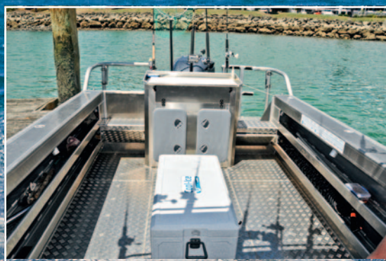
The cockpit's sealed chequerplate decks drain to a sump under the transom locker, from where any water is pumped overboard by a 2000gph bilge pump.
