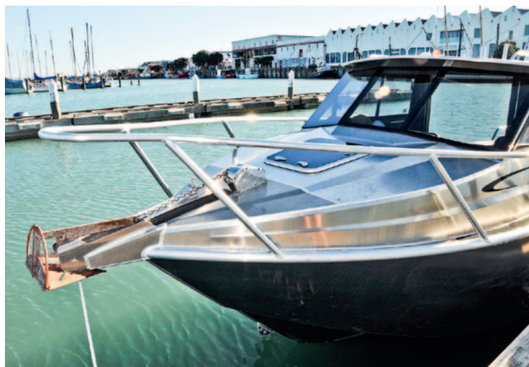
An Anchorlift S912 capstan was mounted on the bow of the big Senator.
