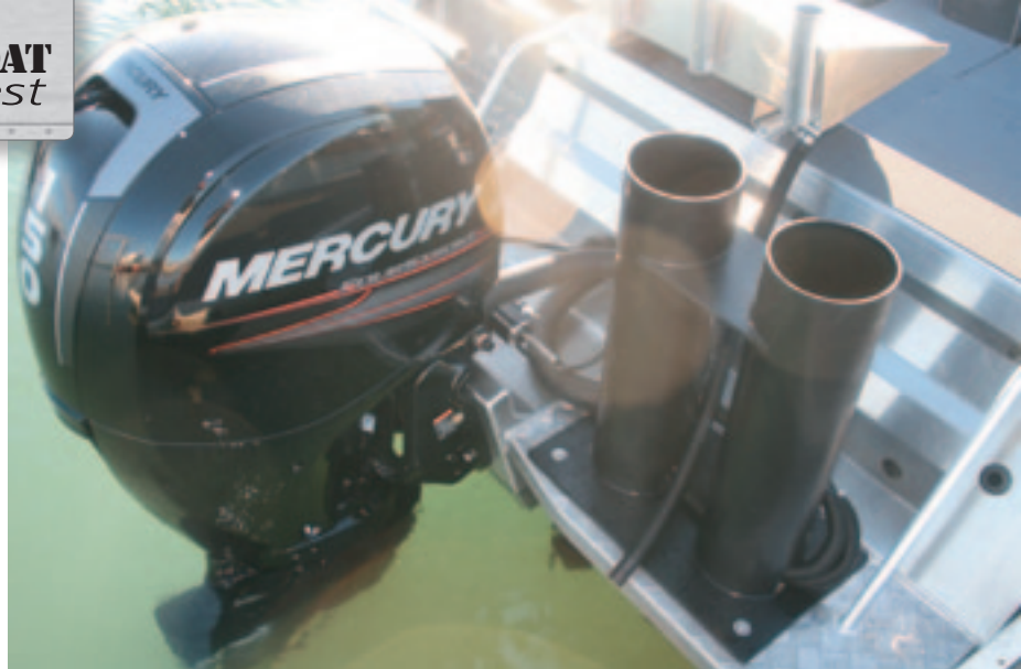
A The Auckland Marine Centre demonstrator had sturdy pair of tuna tubes, complete with external pumps, which can be removed for winter fishing.
