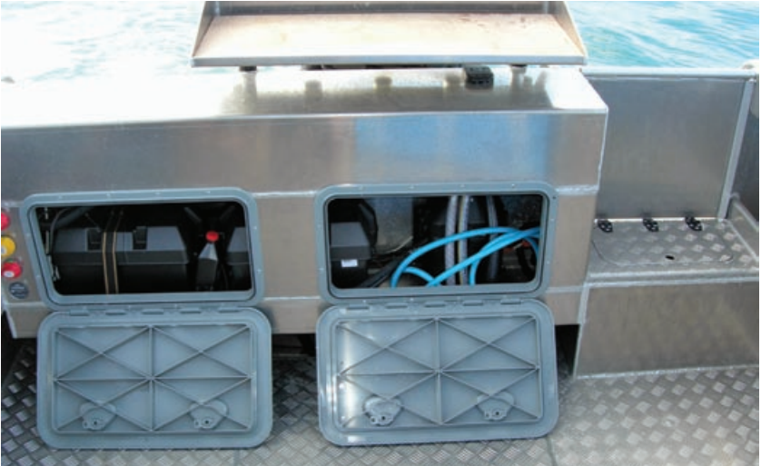
Below: Twin batteries are in a protected position in the transom wall; a live-bait tank is built into the step-through.
