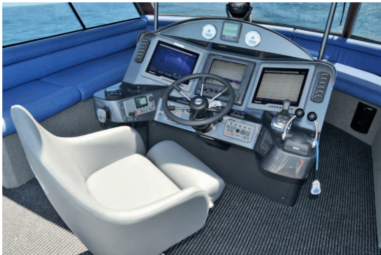
A bit like the helm of the Starship Enterprise. The control station for the Raymarine G-Series electronics is at lower right with the Volvo Joystick control to the right of it.
