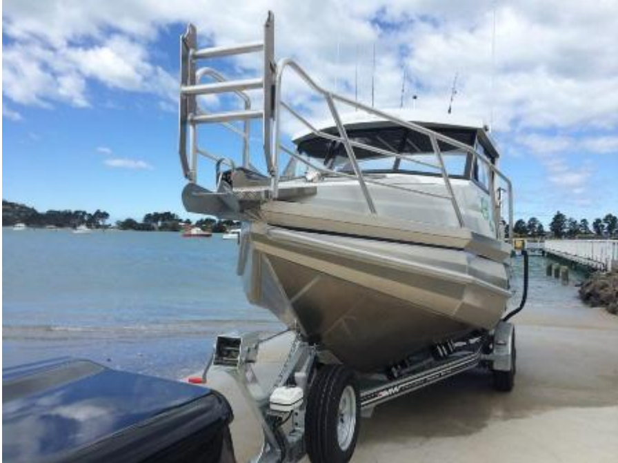
Launching - Bluetooth electronic brakes, boarding ladder, spec'd up DMW trailer
