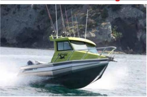
The spacious cockpit and wide top pontoon design are key features, along with the solid construction and stability ensuring a soft ride. The extra buoyancy high in the pontoon sides combined with the multi-chambered construction provides the ultimate in safety. You will be surprised at the features that Senator call standard, the quality of workmanship and the
