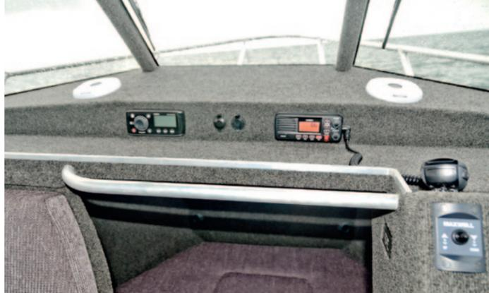
The sound system and VHF are flush-mounted in the dash face.
