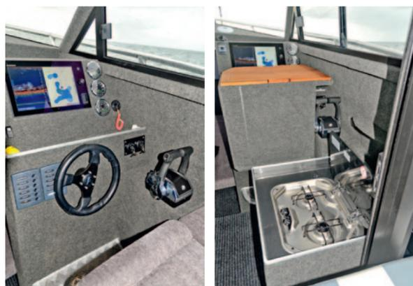
From left: electronic requirements were handled by the latest Furuno Navnet TZ Touch 14 multifunction display. The helm seat folds back to disclose a two-burner cooker and forms a work-top with the addition of a wooden insert.
