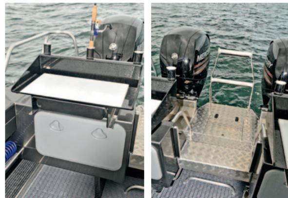
From left: the removable bait stations feature three rod holders, drained rear gutter and stowage tray. A transom step-through makes for easy boarding.
