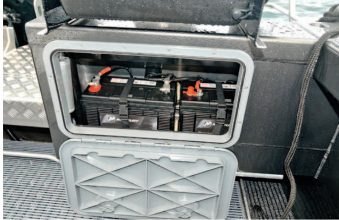
The twin-battery system is in a protected position in a transom locker.
